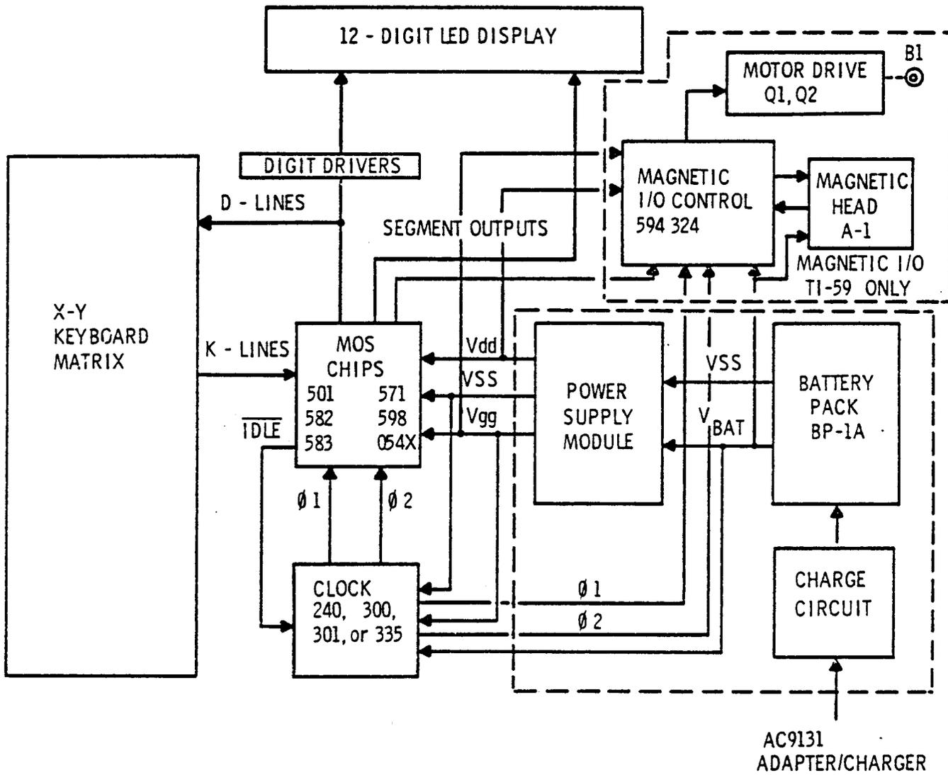
Figure 1. Calculator Block Diagram
