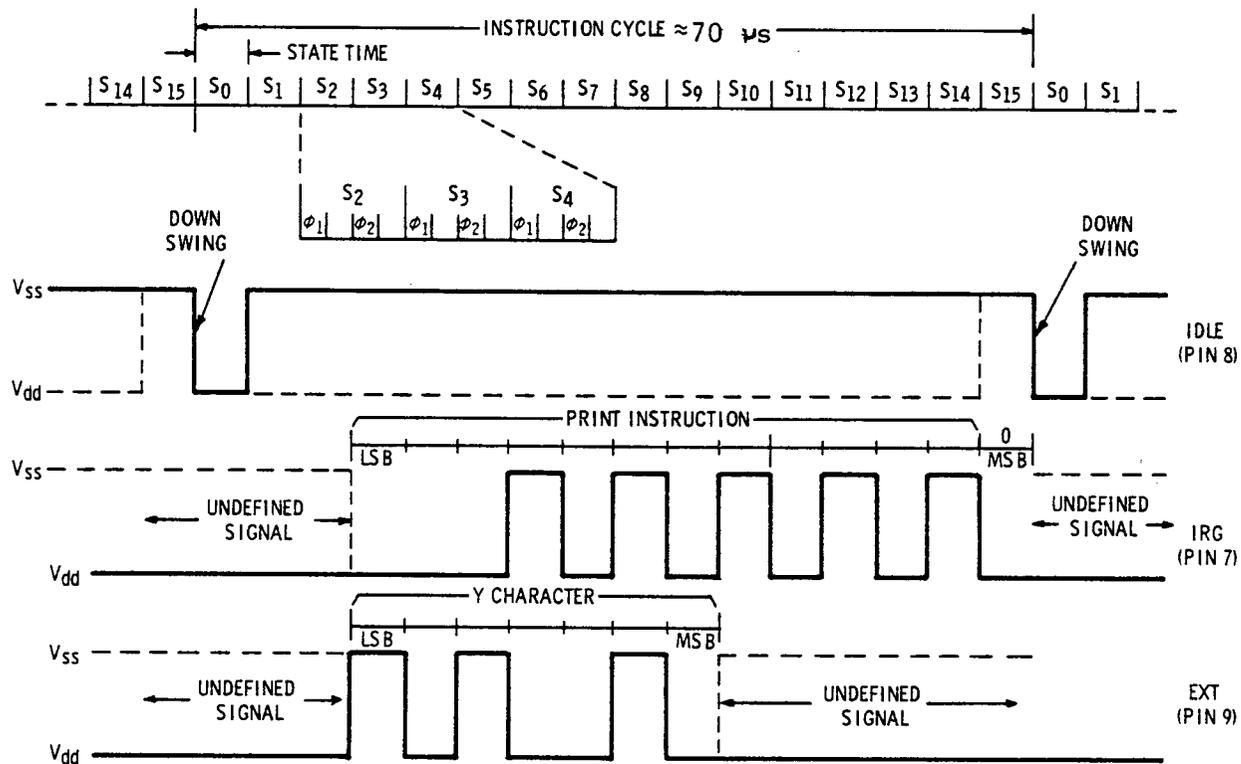
Figure 8. Identification Code Cycle Timing Diagram
