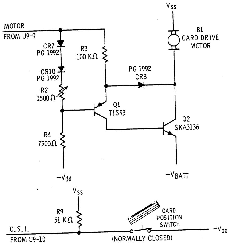
Figure 6. Card Sense Circuit
