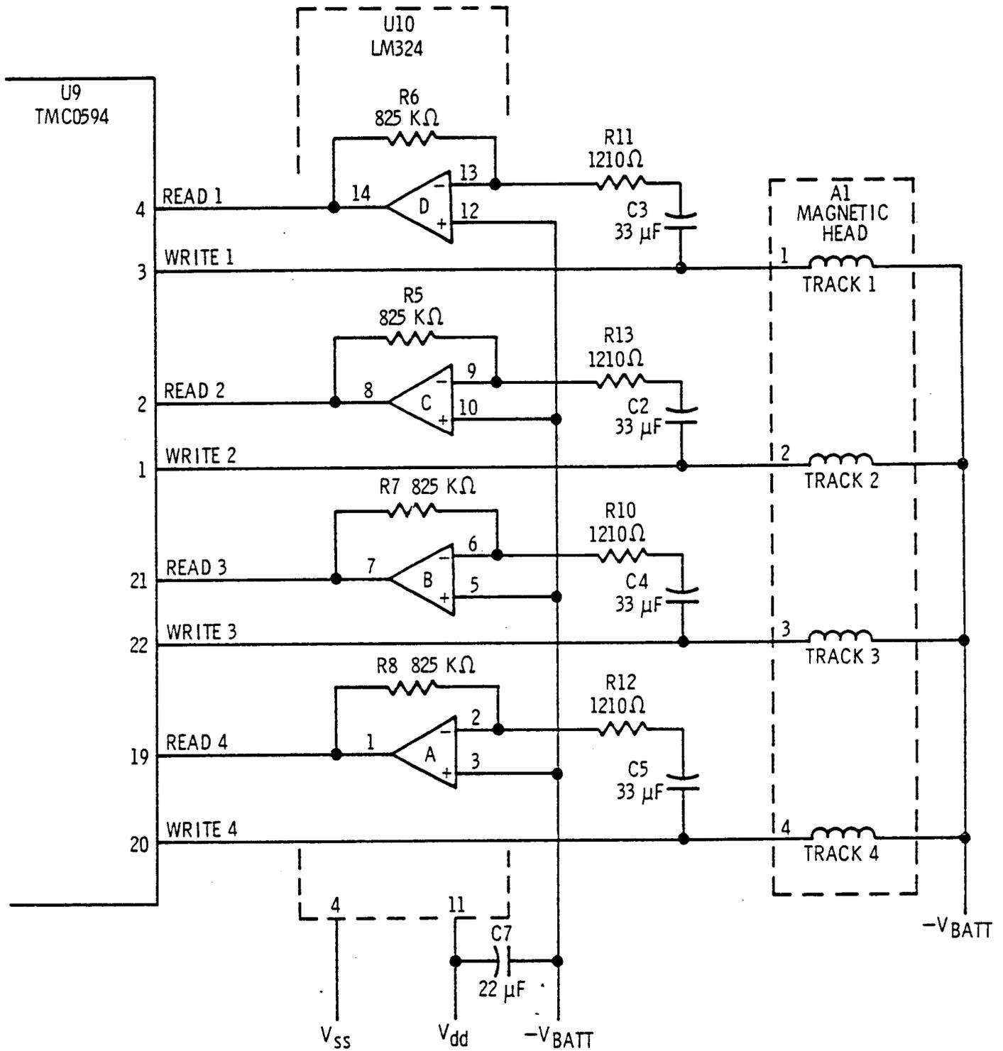
Figure 5. Magnetic Card I/O Circuit
